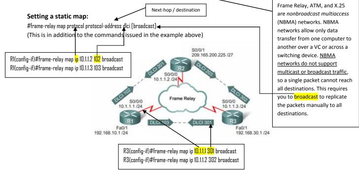
Setting up Frame Relay with subinterfaces:
